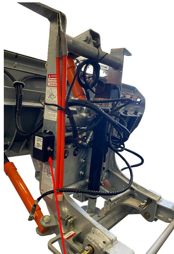
Switch Setup on WING Plow
