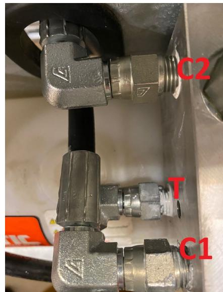
Straight Blade power unit – P &amp; T hose installation
